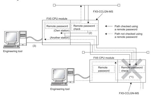
\*1 Since the remote password check is set, the communication request from the external device is not accepted. If the remote password check is not set, the communication request can be accepted and data communications from the external device can be performed.
