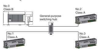
No.0: Master station No.1, No.2, and No.3: Remote station Class A: Authentication Class A device Class B: Authentication Class B device
