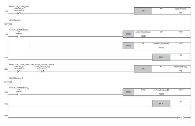
(8) Communication program with the master station (station No.0) (36) Communication program with the local station (station No.2)
