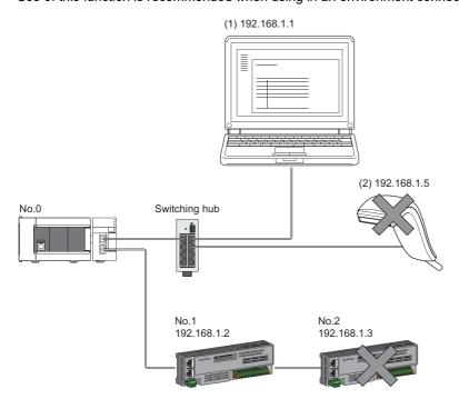
When the "Allow" IP addresses are set to 192.168.1.1 and 192.168.1.2 using the IP filter of the master station No.0: Only the Ethernet device (1) and slave station No.1 can access the master station, and the Ethernet device (2) and slave station No.2 cannot access the master station.
