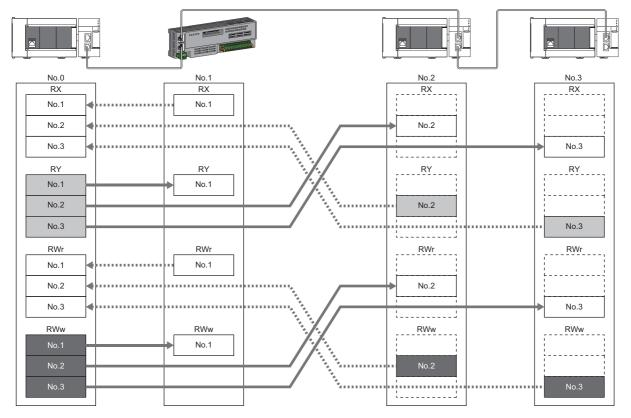
: When the link refresh source is set to a source other than Y, data is held or cleared according to the parameter setting. When the link refresh source is set to Y, data is cleared regardless of the parameter setting.
