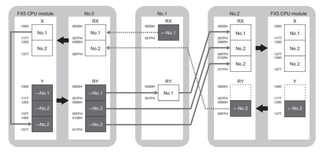
$\rightarrow$ No.1,  $\rightarrow$ No.2: Send range: to station No.1, send range: to station No.2  $\leftarrow$ No.1,  $\leftarrow$ No.2: Send range: from station No.1, send range: from station No.2 9
