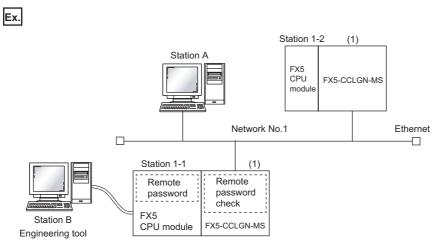
The password can be unlocked and locked by the following external devices.  $\bullet$  1-1 station (1): A station only
