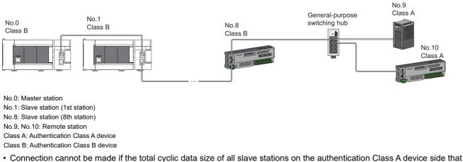
Connection cannot be made if the total cyclic data size of all slave stations on the authentication Class A device side tha form a boundary between authentication Class B and authentication Class A exceeds 2K bytes.
