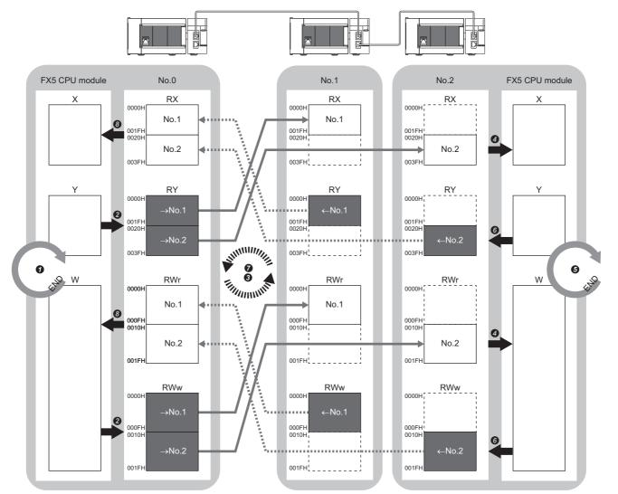
No.0, No.1, No.2: Station No.0 (master station), station No.1, station No.2  $\rightarrow$  No.1,  $\rightarrow$  No.2: Send range: to station No.1, send range: to station No.2
