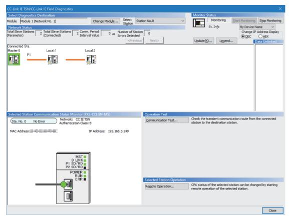
If an error icon appears in "Network Status" area, use the CC-Link IE TSN/CC-Link IE Field diagnostics to identify the cause of the error and take corrective actions. ( Page 144 Checking the Network Status)
