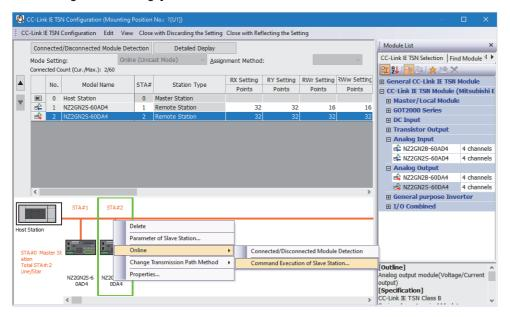
Select and right-click the slave station, select "Command Execution of Slave Station" from "Online" to display the "Command Execution of Slave Station" window.
