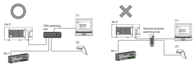
No.0: Master station No.1: Remote station (1), (2): Ethernet device
