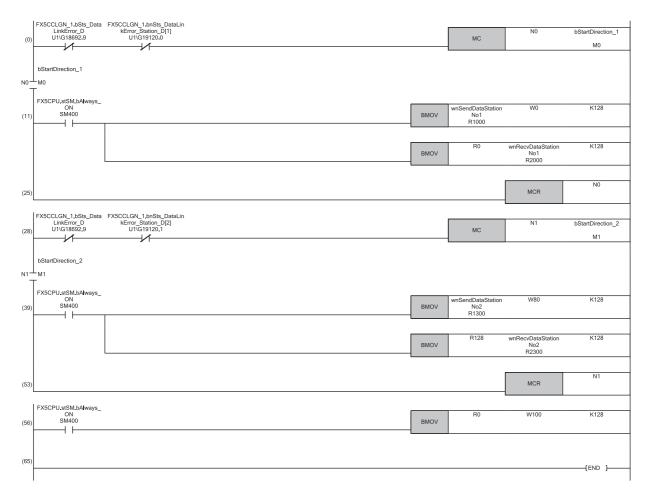
(11) Communication program with the remote station (station No.1)
