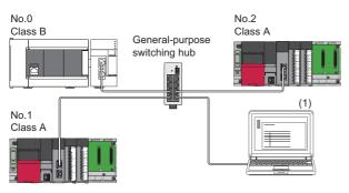
No.0: Master station No.1, No.2: Local station (1) Ethernet device Class A: Authentication Class A device Class B: Authentication Class B device
