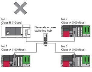
No.0: Master station No.1, No.2, and No.3: Local station Class A: Authentication Class A device Class B: Authentication Class B device • When "Communication Mode" is set to "Multicast" and the communication speed of the master station is set to "1Gbps", slave stations with different communication speeds of 1Gbps and 100Mbps cannot be connected on the end side via a switching hub.
