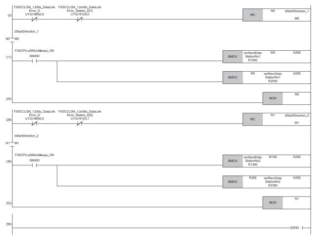
(11) Communication program with the local station (station No.1)(39) Communication program with the local station (station No.2)
