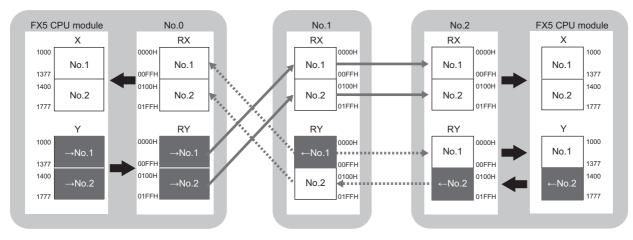
$\rightarrow$ No.1,  $\rightarrow$ No.2: Send range: to station No.1, send range: to station No.2  $\leftarrow$ No.1,  $\leftarrow$ No.2: Send range: from station No.1, send range: from station No.2
