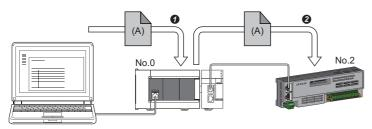
Save parameter (A) of the slave station to the FX5 CPU module in the master station. When the slave station is returned/connected, saved parameter (A) is automatically set from the master station to the slave station.
