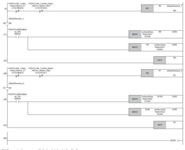
(11) Communication program with the local station (station No.1)(39) Communication program with the local station (station No.2)
