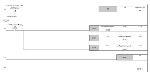
(8) Communication program with the master station (station No.0) and the remote station (station No.1)
