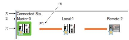
Displays the station (own station) where the engineering tool is connected.
