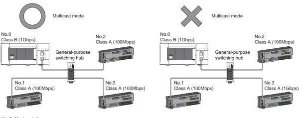
No.0: Master station No.1, No.2, and No.3: Remote station Class A: Authentication Class A device Class B: Authentication Class B device
