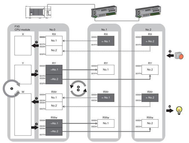
No.0, No.1, No.2: Station No.0 (master station), station No.1, station No.2
