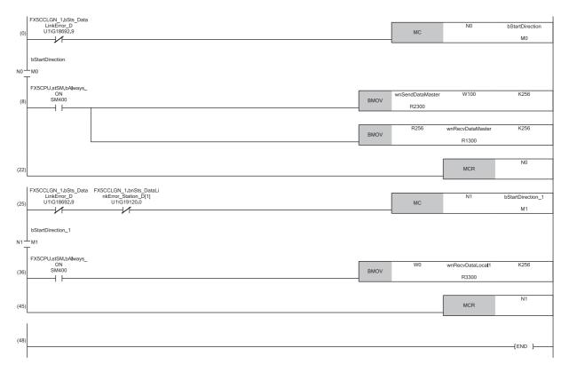
(8) Communication program with the master station (station No.0)(36) Communication program with the local station (station No.1)
